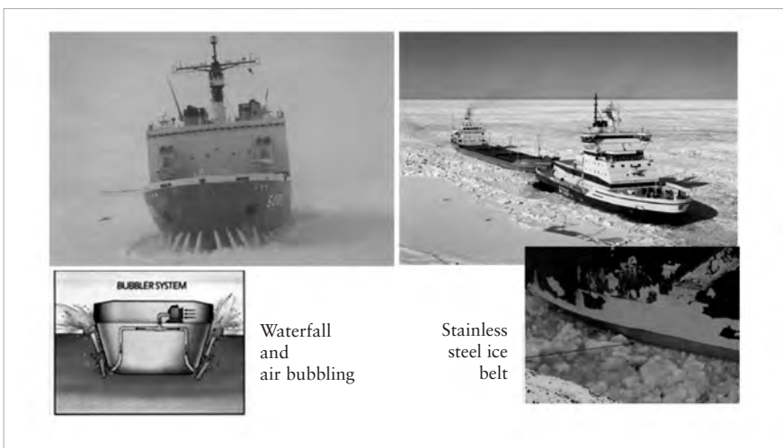
Figure IV-14. Examples of typical additional features for friction reduction for ice-going ships
