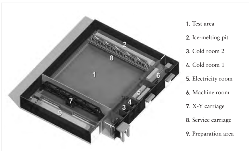
Figure IV-4. Layout of KRISO Ice Tank
