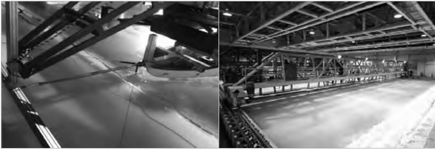
Figure IV-5. X-Y carriage and service carriage
