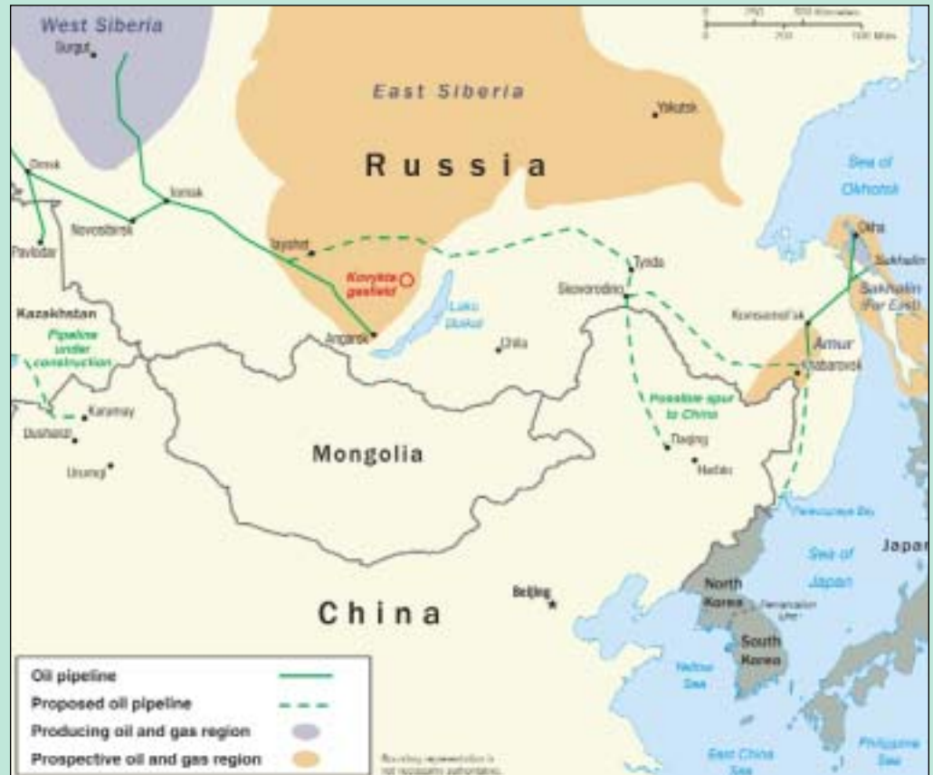
Proposed route of oil pipeline from Taishet, northwest of Lake Baikal, to Perevoz-naja Bay on the Pacific coast of the Russian Far East, with a spur line to Daqing in northeastern China. Source: EIA (2006).
