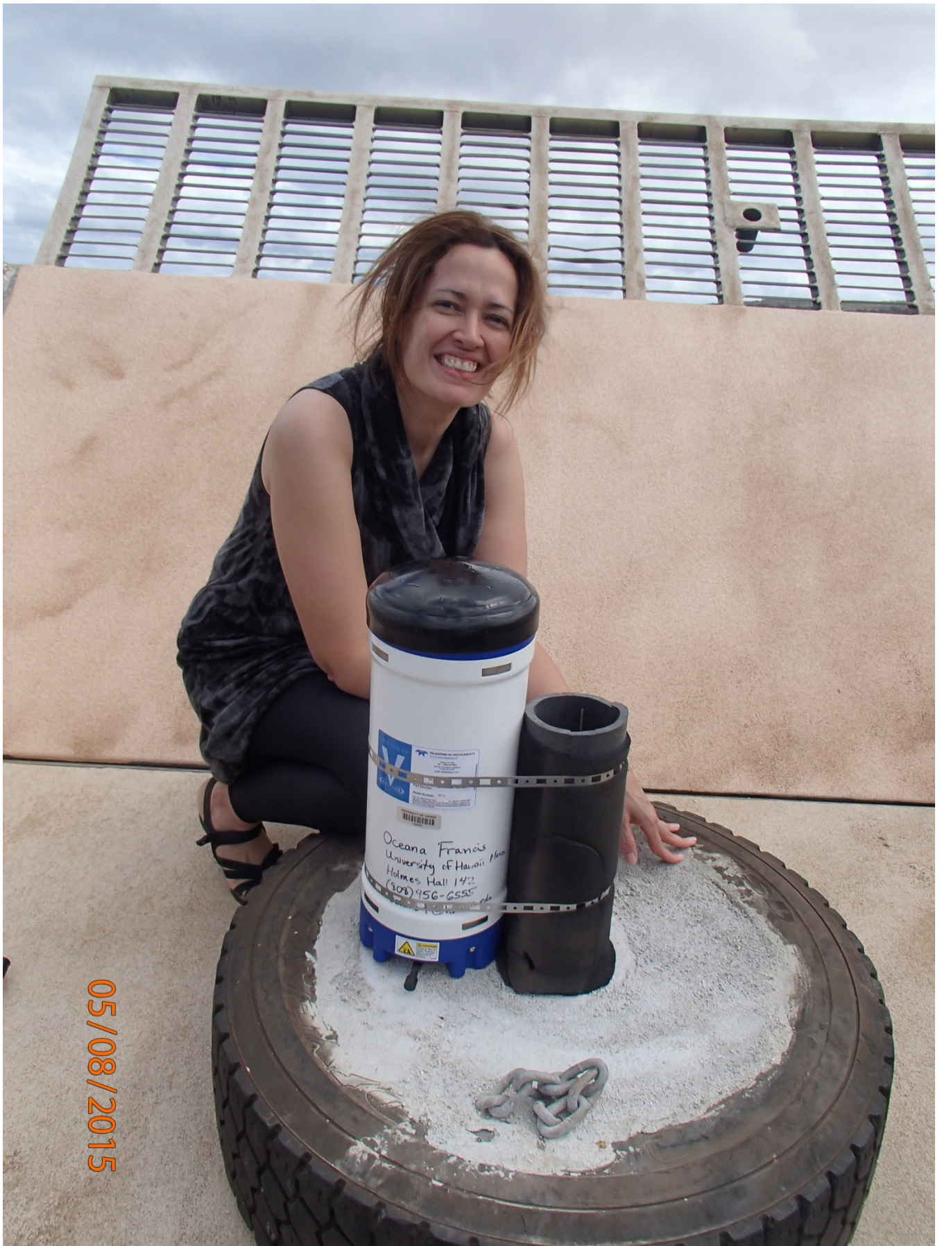
Dr. Francis deploying an ADCP from her lab which measures full wave spectrum and current velocity profiles off the coast of Kahoolawe.
